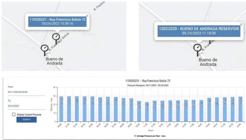
Figure 9: Pressure control point in the distribution network
